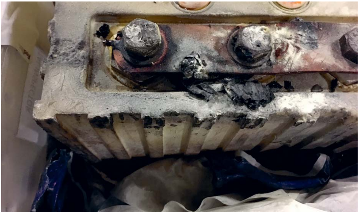
Lithium battery fire in a postal item.
