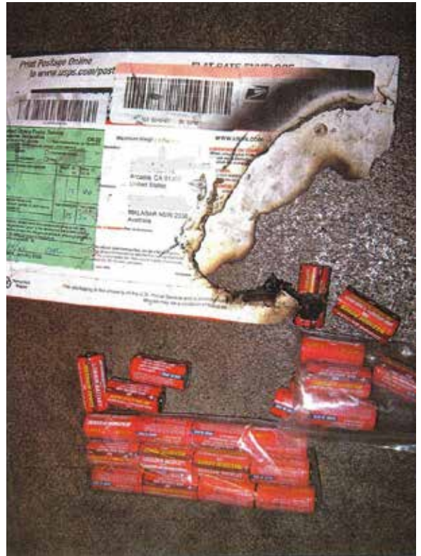
Damage caused by lithium batteries (Photo: USPS)
